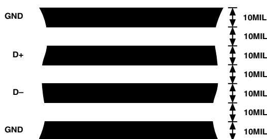
Figure 6. Arrangement of Signal Tracks
